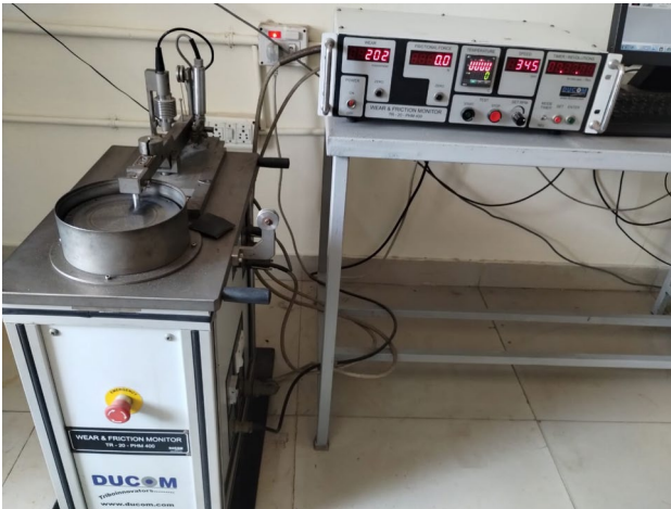
Fig. 5 Ducom made pin-on-disc wear test apparatus
